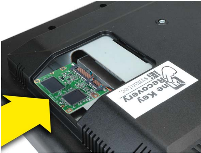
Figure 3-2: SATA DOM Card Installation
